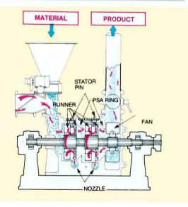
The Super Micron Mill is a 2-chambered fine pulverizer which employs 2 sets of runners revolving on a central shaft. These runners consist of a No.1 and No.2 in each chamber to which are fastened special alloy tips. In addition to these runners are grooved liners and 4 adjustable stator pins in each chamber. For the purpose of having horizontal air flow in the chambers and to convey finely pulverized particles, an impeller fan is located immediately
