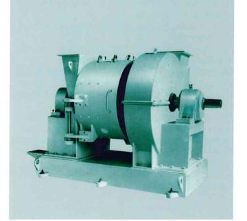
The Fine Micron Mill is basically a high speed air swept type impact mill and come with three different models, but has a new unique and proven concept of the grinding mechanism originated through long and continued research and development works. This mill is suited for ultra fine grinding at a large capacity especially for talc, limestone and other non-ferrous mineral ores.
