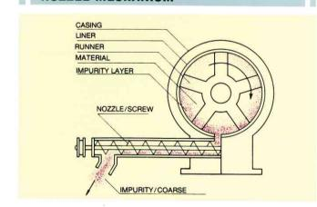
The impurities are extracted by the nozzle so that high quality of products are obtained. As shown in the figure, the impurities separated from ground material normally have higher specific gravity and coarser size, thus they receive higher centrifugal force by grinding hammers. Therefore these particles are pressed against inner circumference of the milling chamber, thrown into the nozzle inlet and discharged outside.
