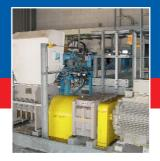
Natural and synthetic rubbers are usually delivered in 'bales'. These have to be size reduced to facilitate blending with other ingredients or dissolving. The size of the machine required is determined by the thickness of the bale and the customer's throughput requirement –
