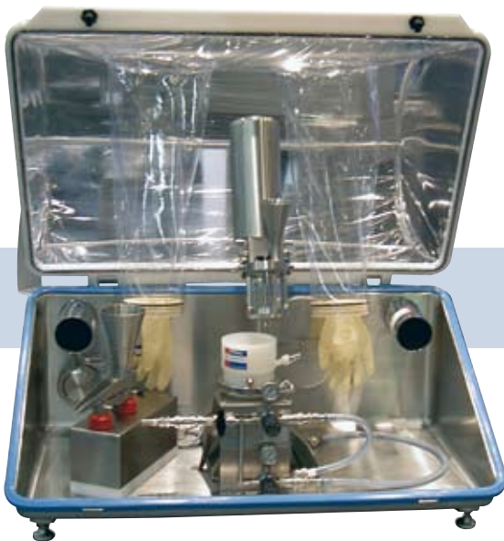
FLEXIBLE ISOLATOR (OEL < 10 µg/m 3 ) WITH DISPONABLE MODEL OF 50 AS IN PVDF
